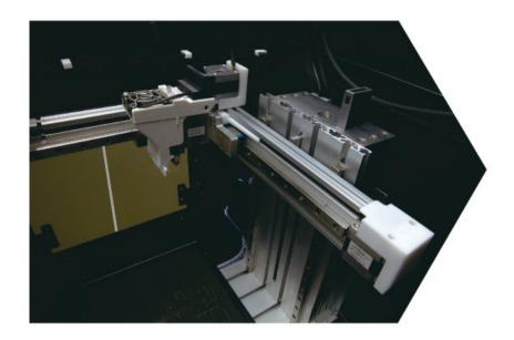
The X5 is a breakthrough in 3D printing, designed from the ground up for low-volume manufacturing. Capable of automatically feeding up to 12 print beds onto its build plate and reloading during printing, it provides a continuous 3D printing experience.
